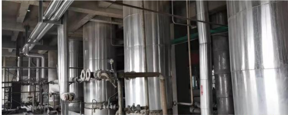
Potassium nitrate production line of 170,000 tons / year using ion exchange process (high standard molten salt material) )
