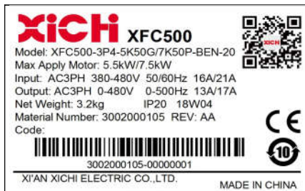
Fig. 2-2 Description of frequency converter's nameplate
